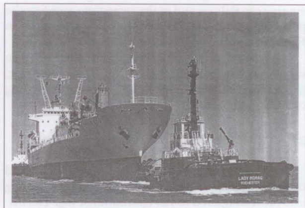
Figure 8 - ASD - tug in typical manoeuvre
