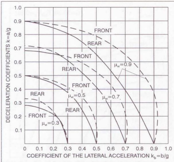
Figure 4 - Road-holding limits of the front and rear wheels of a ready-for-movement vehicle at various conditions of the road surface for the installed braking system with bi-linear characteristics
