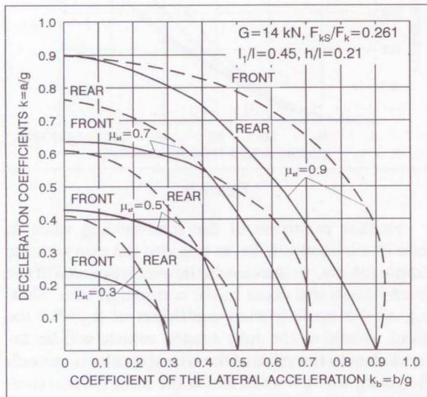
Figure 2 - Limits of road-holding features of the front and rear wheels in ready-for-movement condition with various road surface conditions for the installed braking system with linear characteristic
