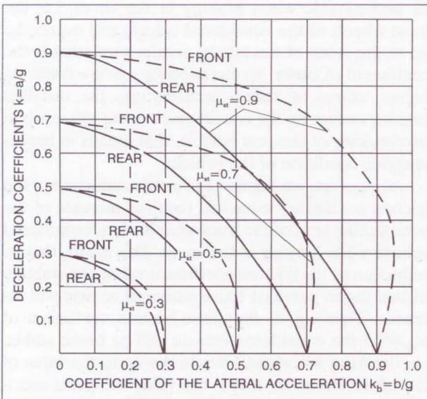
Figure 5 - Road-holding limits of the front and rear wheels of a ready-for-movement vehicle at various road surface conditions for the braking system with the ideal distribution of braking forces per vehicle axes.
