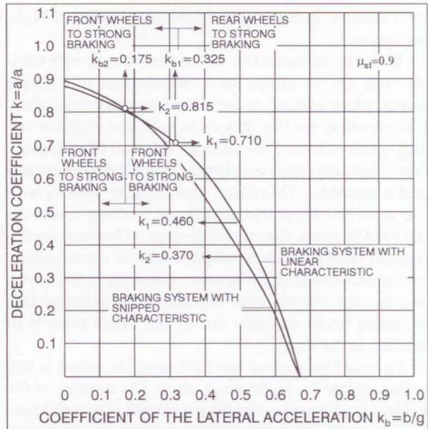
Figure 9 - Functional dependence between slowing down and lateral acceleration of the vehicle at the road-holding limit for the installed braking system with a linear characteristic and with a bilinear characteristic.
