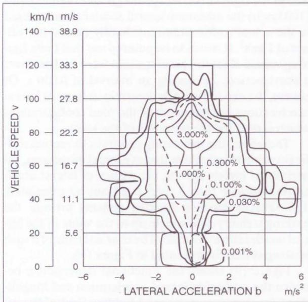
Figure 8 - The frequency of lateral accelerations in studying the vehicles in actual traffic situations
