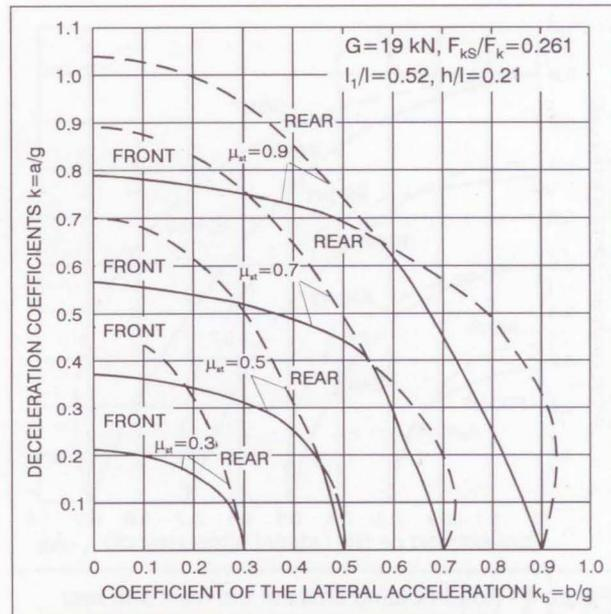
Figure 3 - Road-holding limits of the front and rear wheels of a fully loaded vehicle in different road surface conditions for the installed braking system with linear characteristic.
