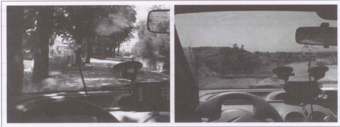
Figure 7 - The installation of a visual stimulator in the direct line of sight (left, avoidance to the left is stimulated) and off-center to the line of sight (right, extreme braking is stimulated) for the real driving environment experiment
