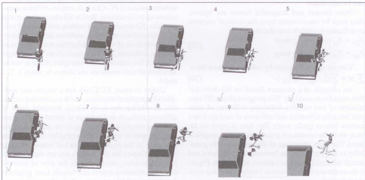
Plate 4 - PC-Crash simulation of a vehicle-cyclist collision at vehicle speed of 40 km/h, and cyclist speed of 10 km/h.
