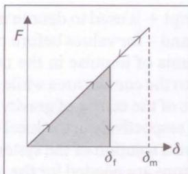
Figure 3 - The force-deflection relationship where  $\delta_f$  is the final (residual) deflection,  $\delta_m$  is the maximum deflection
