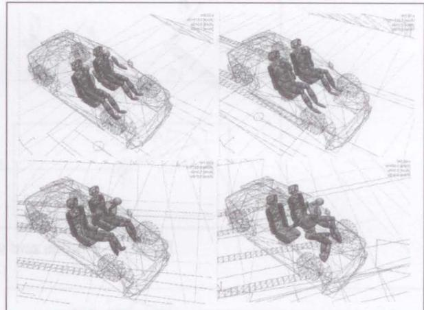
Plate 2 - The PC-Crash simulation of an occupant's motion before impact after skidding with locked wheels; interval between frames is 0.5 s.
