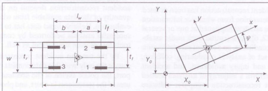
Figure 1 - The variables of vehicle dimensions and position
