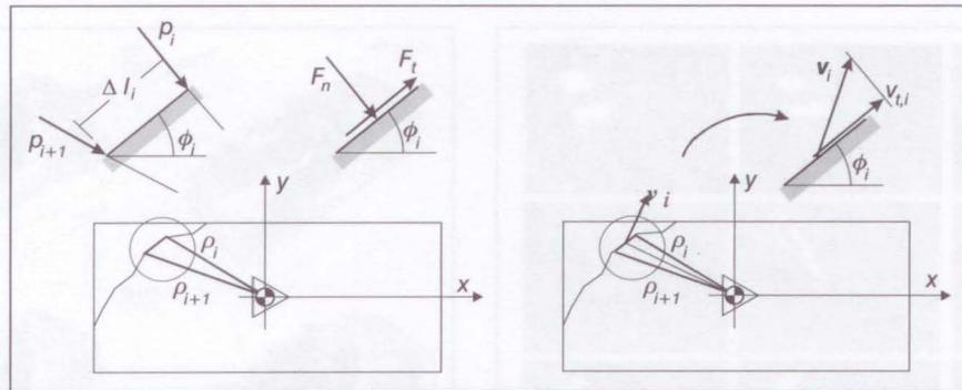
Figure 5 - Forces and velocity at crushed segment
