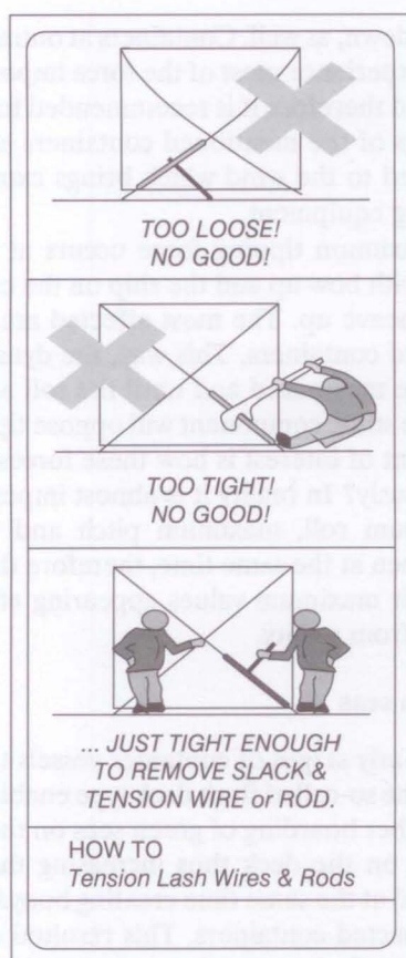
Figure 5 - Proper lashing
