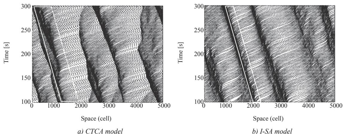
*Figure 1 – Spatial-temporal diagram of the CTCA model and the I-SA model with density of 40 veh/km*
