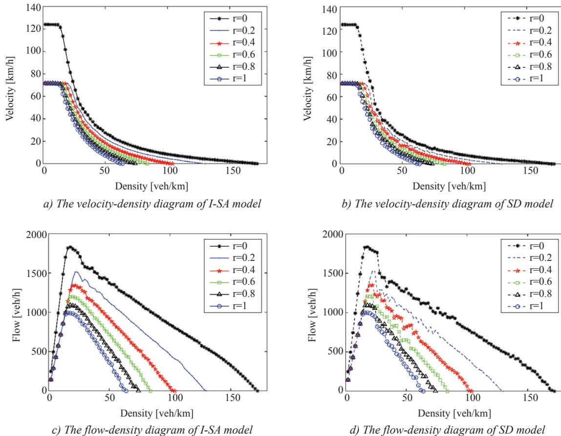
Figure 4 – The fundamental diagrams
