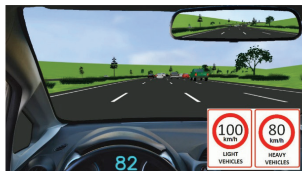
Figure 3 – Driver's view of the road and surrounding landscaped area through the windshield, with speed indication (in km/h) on the dashboard and a traffic stream presenting a density of 16.8 veh/km/lane
