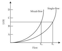
Figure 7 – Relationship between flow and LOS
