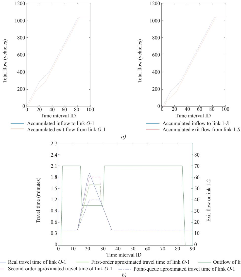
Figure 5 – a) Cumulative Inflow of O-1 and Exit Flow Curves 1-S; b) Travel Times and Exit Flow Rate of Link O-1 with Inflow Rate of 4200 vph
