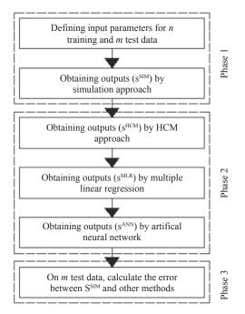
Figure 1 – Modelling phases in the estimation of saturation flow rate
