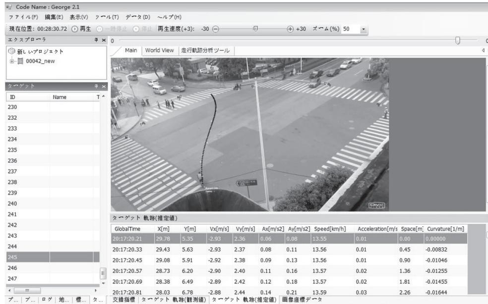
Figure 4 – Movement of vehicles analysed by George 2.1
