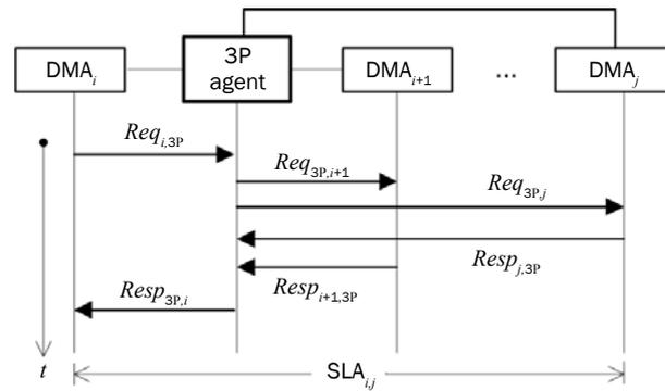
Figure 3 – The single signalling transaction via 3P agent
