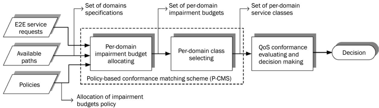
Figure 6 – SEA prototype: Service negotiation flowchart
