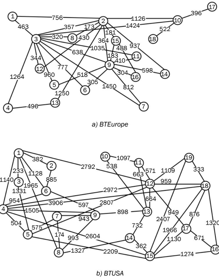
Figure 4 – Simulated network topologies (the numbers on the links represent air distance in kilometres)
