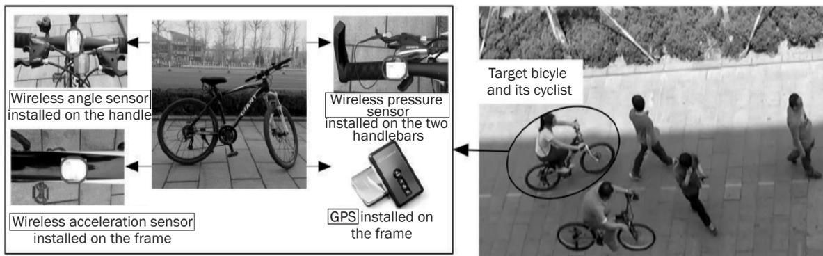
Figure 4 – Dynamic acquisition system for complex information of bicycle and its cyclist
