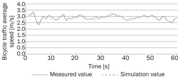
Figure 9 - Simulation verification for average speed
