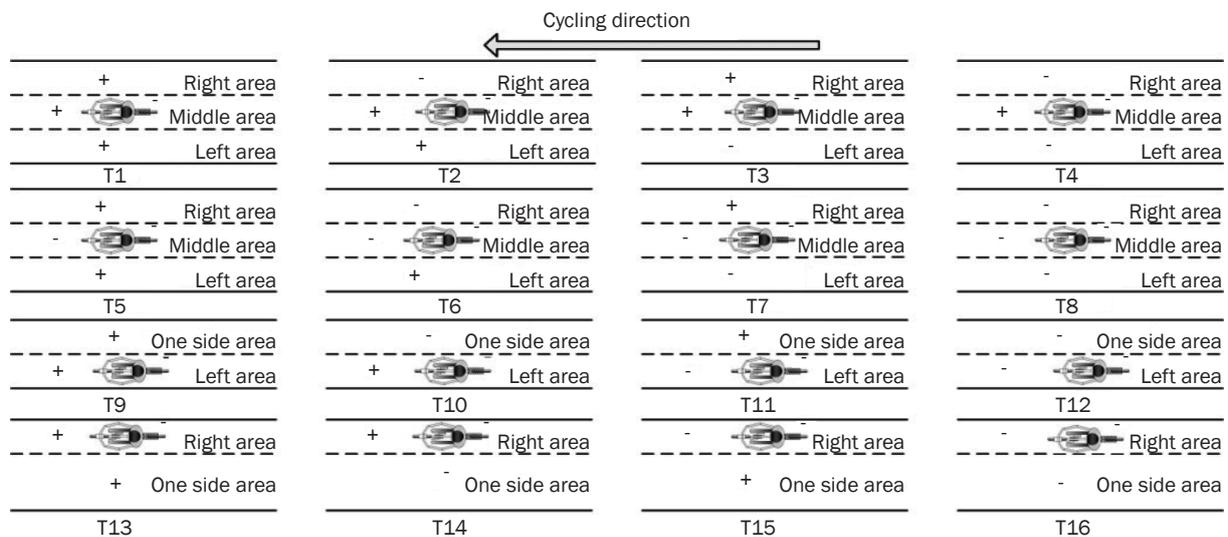
Figure 2 – Simple pedestrian-bicycle traffic phase
