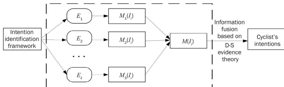
Figure 3 – Cyclist's intention identification model based on D-S evidence theory
