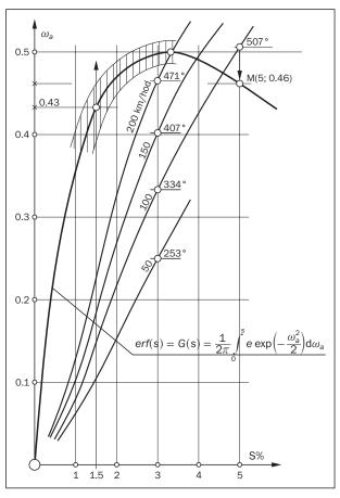
Figure 1 - Theoretical prediction of the contact temperatures T, drawn along the slip curve
