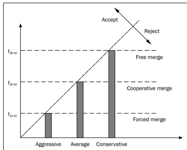
Figure 2 - Acceptable headway for different types of drivers
