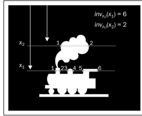
Figure 4 – Example of determination of  $inv_{h,i}(x)$
