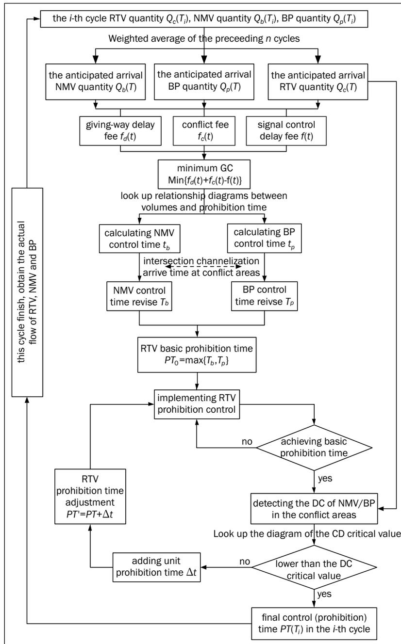
Figure 6b - The detailed RTV signal control flowchart
