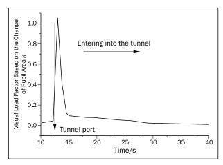
Figure 5 - Visual load factor based on the change of pupil area along tunnel road
