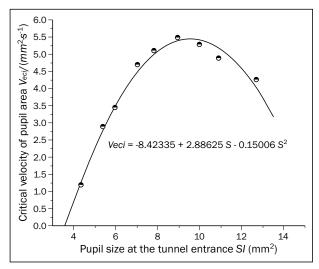
Figure 4 - Correlation between pupil area and its critical velocity at tunnel entrance
