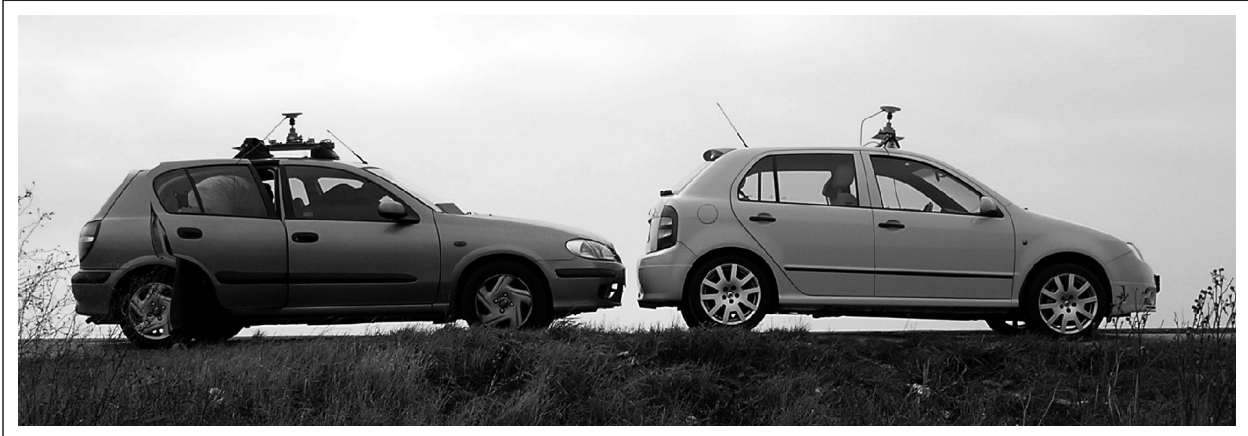
Figure 1 - Photo of GPS antennas that are placed on the strap on the top of the vehicle. (Photographed during steady measurement of minimal vehicle distance)
