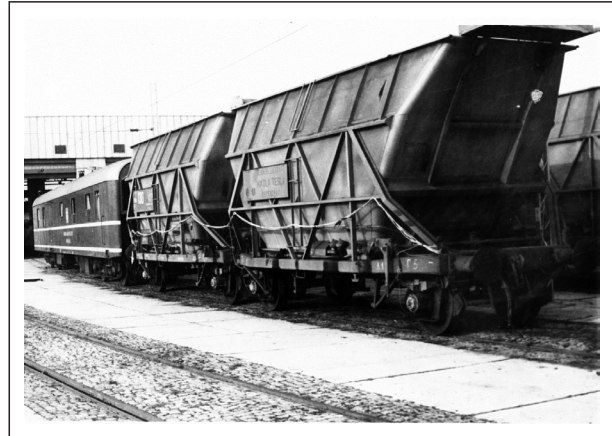
Figure 1 - Four-axle double wagon Fbd for coal transport
