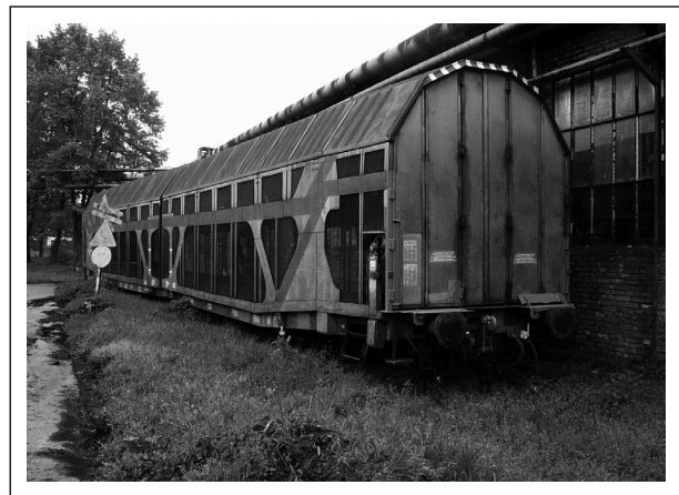
Figure 2 - Three-axle DDam car transport wagon
