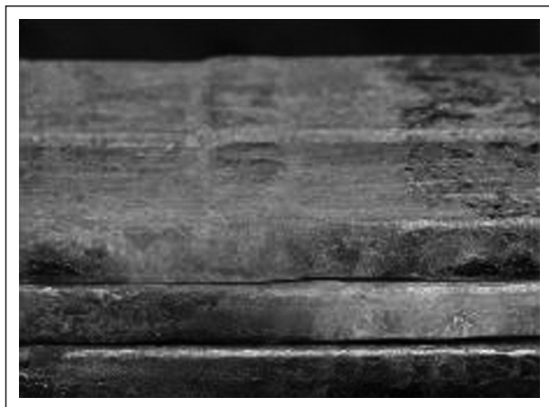
Figure 7 - Welded main leaf of the spring
