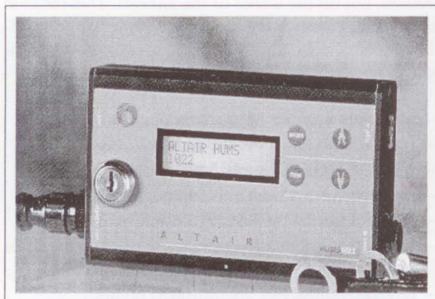
Figure 1 - Control box HUMS Altair 1022 on-board aircraft
