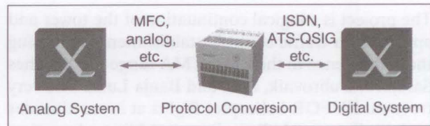
Figure 7 - Communication systems with different protocols can be integrated via Protocol-converter node
