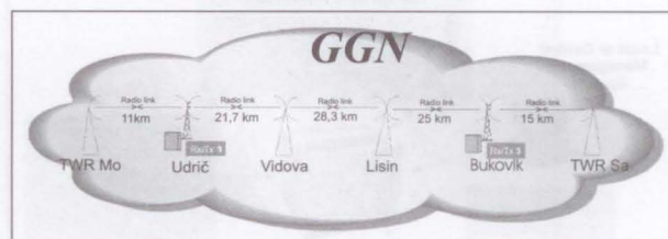
Figure 4 - Radio link connection between Mostar and Sarajevo control tower
