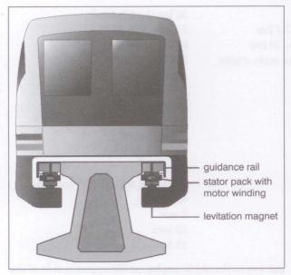
Figure 5 - Cross section
