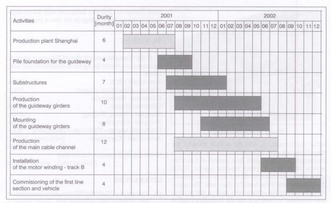
Figure 12 - Planned realization periods of main guideway components
