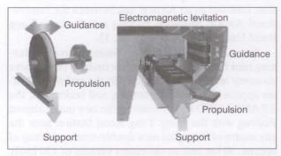
Figure 2 - Levitation and propulsion
