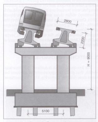
Figure 8 - Cross section
