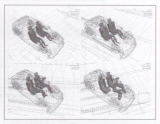
Plate 2 - The PC-Crash simulation of an occupant's motion before impact after skidding with locked wheels; interval between frames is 0.5 s.
