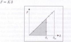
Figure 3 - The force-deflection relationship where  $\delta_{\rm f}$  is the final (residual) deflection,  $\delta_{\rm m}$  is the maximum deflection
