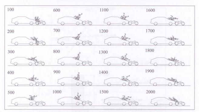
Plate 5 - Working-Model simulation of a vehicle collision into a motorcycle, the simulation of the motorcycle driver and the passenger motion after the initial impact of a vehicle (vehicle speed is 72 km/h, while the motorcycle speed is 36 km/h; intervals between frames are in μs)
