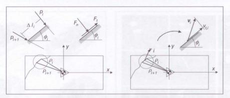
Figure 5 - Forces and velocity at crushed segment
