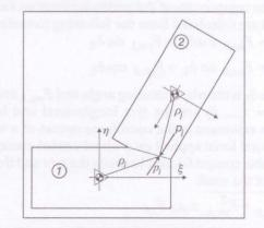
Figure 4 - Computing the crush pressure
