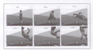
Plate 3 - PC-Crash simulation of a pedestrian's rebound from a car hood shown from the driver's perspective
