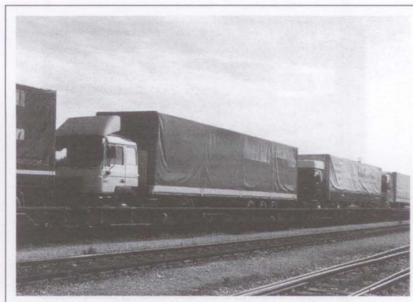
Figure 1 - Wagons for loading of trucks, trucks with trailers and tractors with semi-trailers
