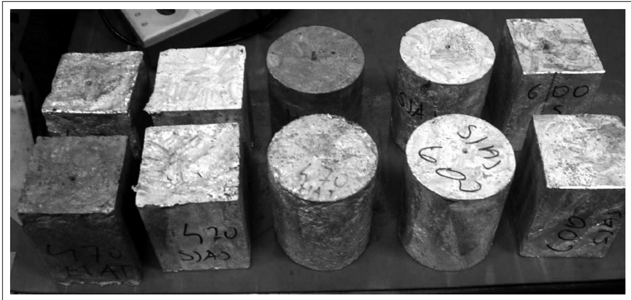
Figure 8 – Aluminium foam samples with different densities and wall materials
