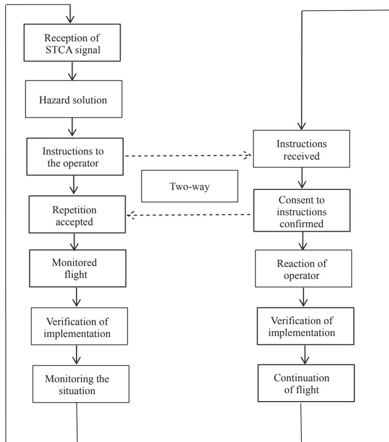
Figure 1 – Flow diagram of the collision hazard signalling and monitoring of a pair of drones
