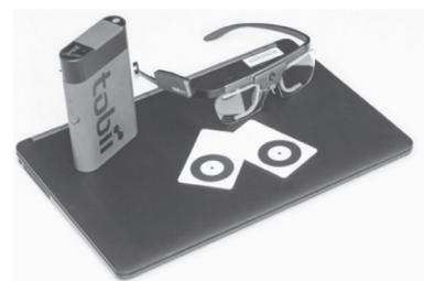
Figure 2 – Elements of a Tobii Pro Glasses 2 eye-tracking system [29]
