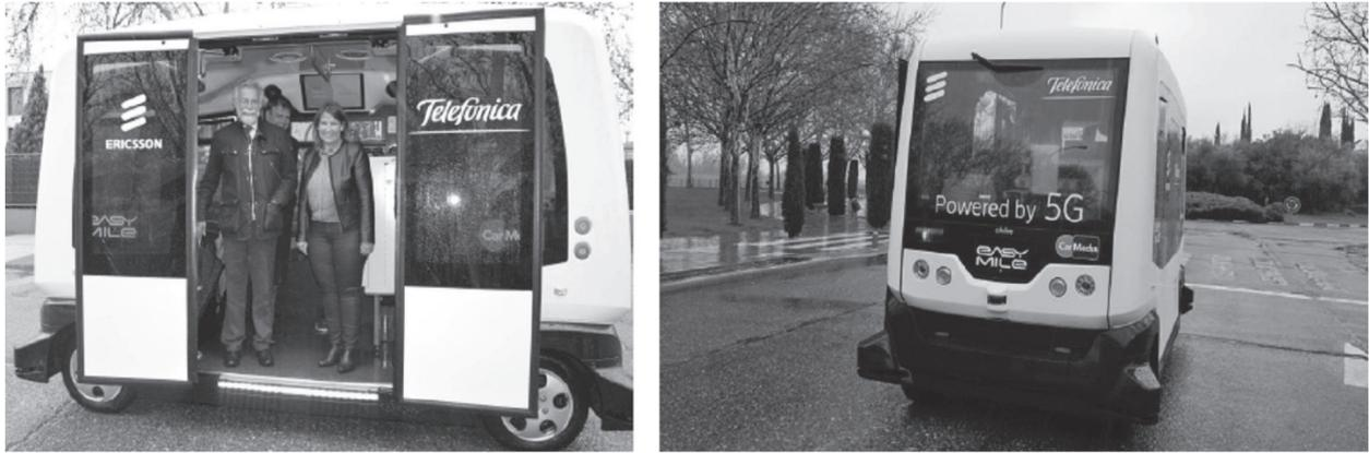
Figure 1 – An example autonomous personal transit system with Ericsson 5G terminal and information platform
