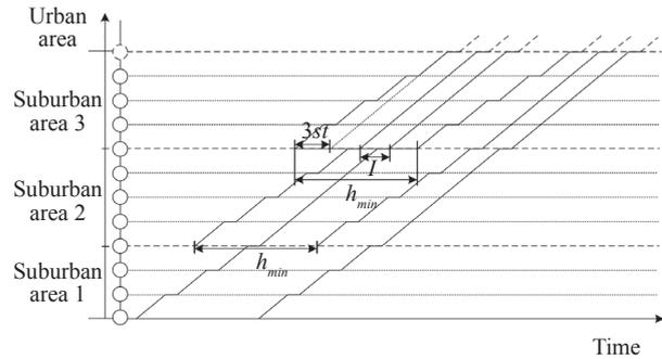
Figure 3 – Diagram of the passing through capacity of the zonal operation mode
