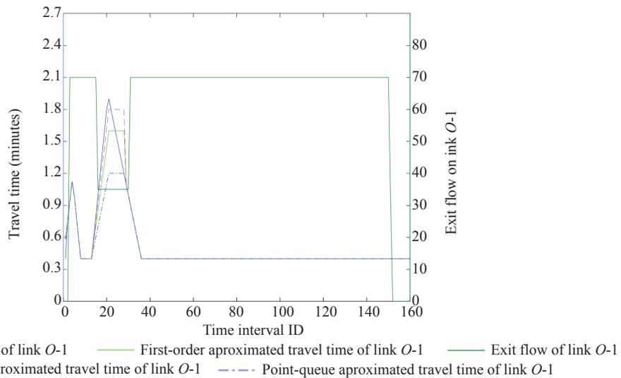
Figure 6 – Travel Times and Exit Flow Rate of the Link (O,1) with an Inflow Rate of 8000 vph
