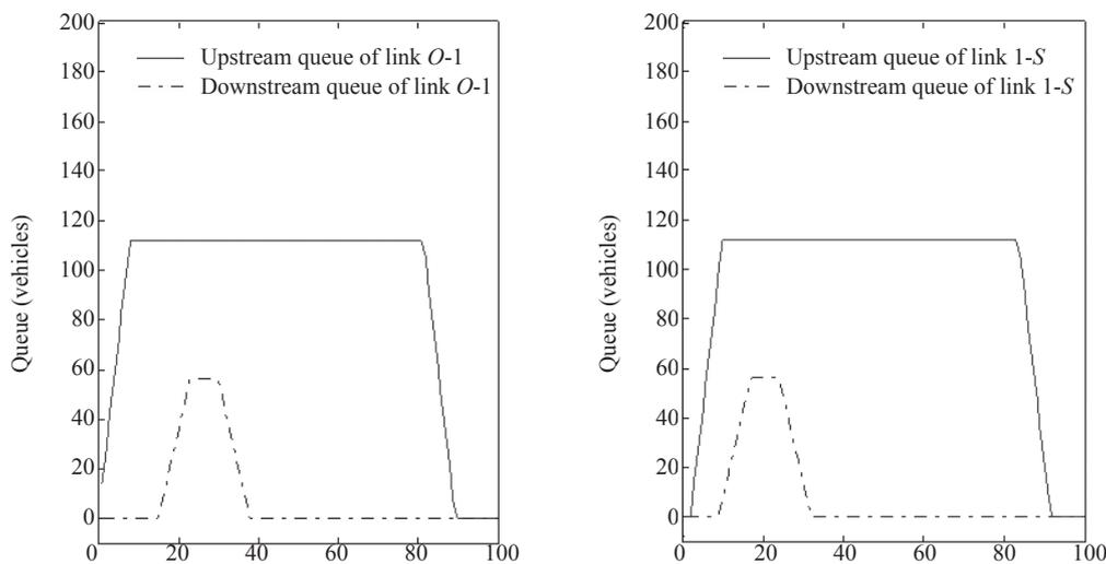
Figure 4 – Upstream and Downstream Queues with Inflow Rate of 4200 vph
