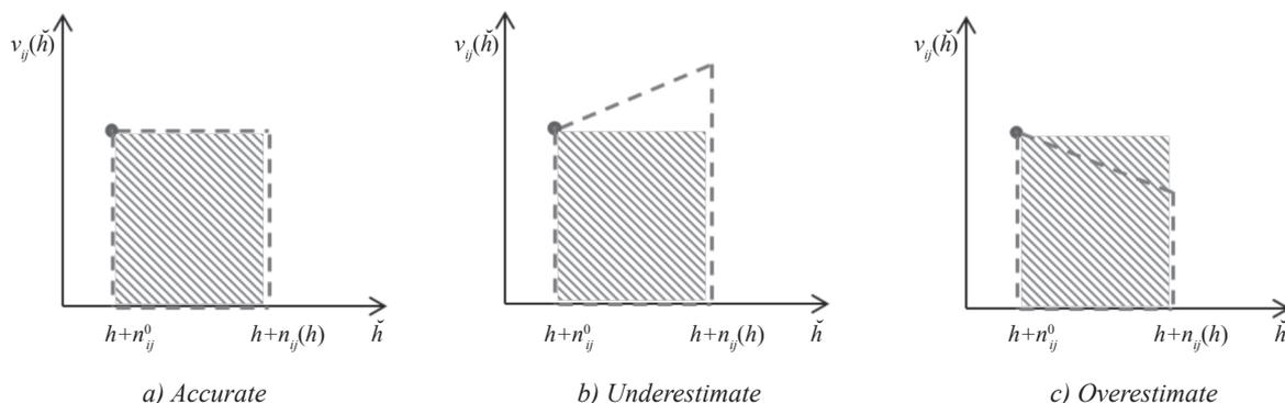
Figure 2 – Link Downstream Queue Approximation
