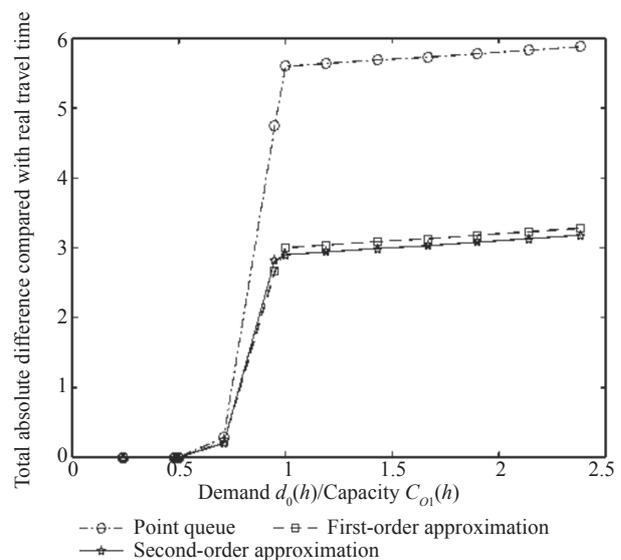
Figure 7 – Total Absolute Difference Compared with Real Travel Time
