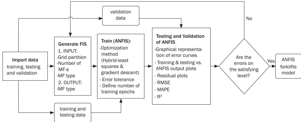
Figure 3 – Methodology steps for building the ANFIS model
