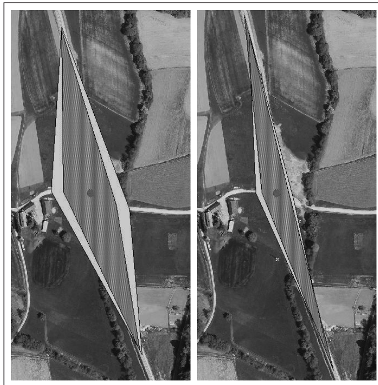
Figure 6 - Comparison between "legislation" and suggested method for defining the visibility field on passive protected level railroad crossings (brighter: suggested method, darker: "legislation" method, left: V_R = 50 km/h, right: V_R = 30 km/h)
